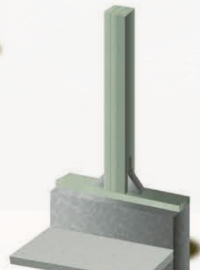
Post on Foundation Wall
