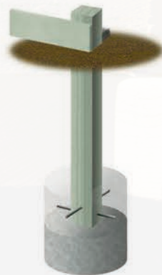
Post with Concrete Collar and Rebar
